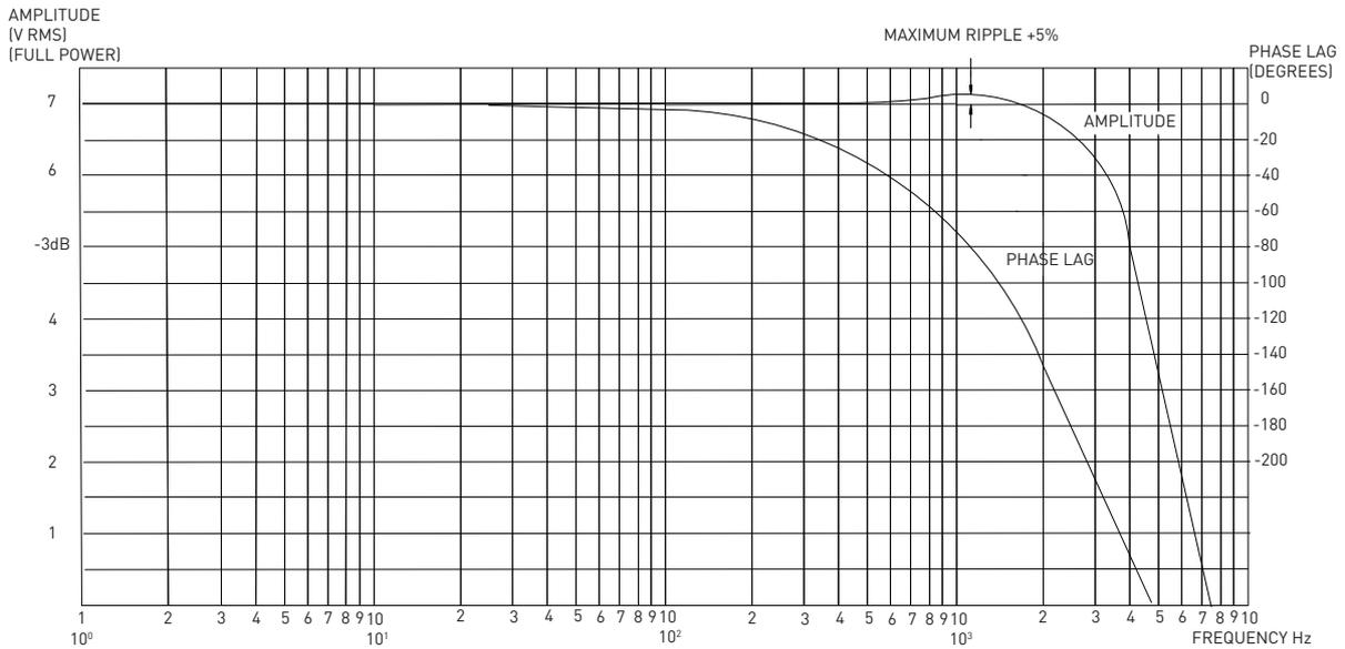
Figure 1: Typical frequency dependent amplitude and phase response
